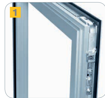
1 Corner drive with mishandling device and incorporated night ventilation.
