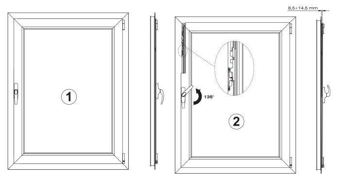
With the leaf in closing position (image 1), turn the handle of 135° (image 2) to obtain the night ventilation opening.
