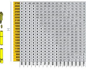
Leaf max weight of 70 Kg for internally flush profiles (art. 3200.740/.742/.743R/.743L/.745)
